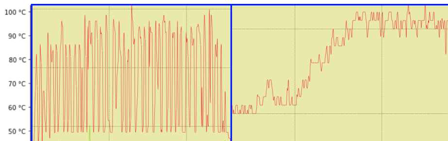
Fig. 3: The CPU temperature time series by sleep injection (left) vs DVFS (right). The x-axis is the time frame and the y-axis is the CPU temperature ranging from 48 °C to 100 °C.
