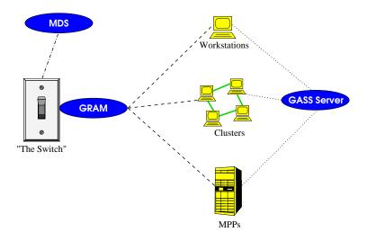
Figure 5: **Ramsey Number application on the Globus infrastructure.** Depicted is the relationship between the Ramsey Number Search application control site, the Grid resources, and the Globus subsystems used. The following Globus mechanisms used by the application and EveryWare toolkit are shown: Globus Resource Allocation Manager (GRAM) the Global Access to Secondary Storage (GASS), and the Metacomputing Directory Service (MDS).
