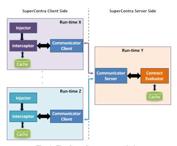
Fig. 1: The SuperContra system design
