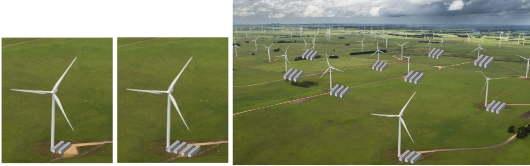
Figure 4. Scaling from Small : 2-container, 2.2 Petaflops, 0.59MW, Medium : 4-container, 4.4 PF both can be power by a single turbine. Extreme : 42-container, 45.5 PF, 12.4MW, 5% of turbines in a wind farm.
